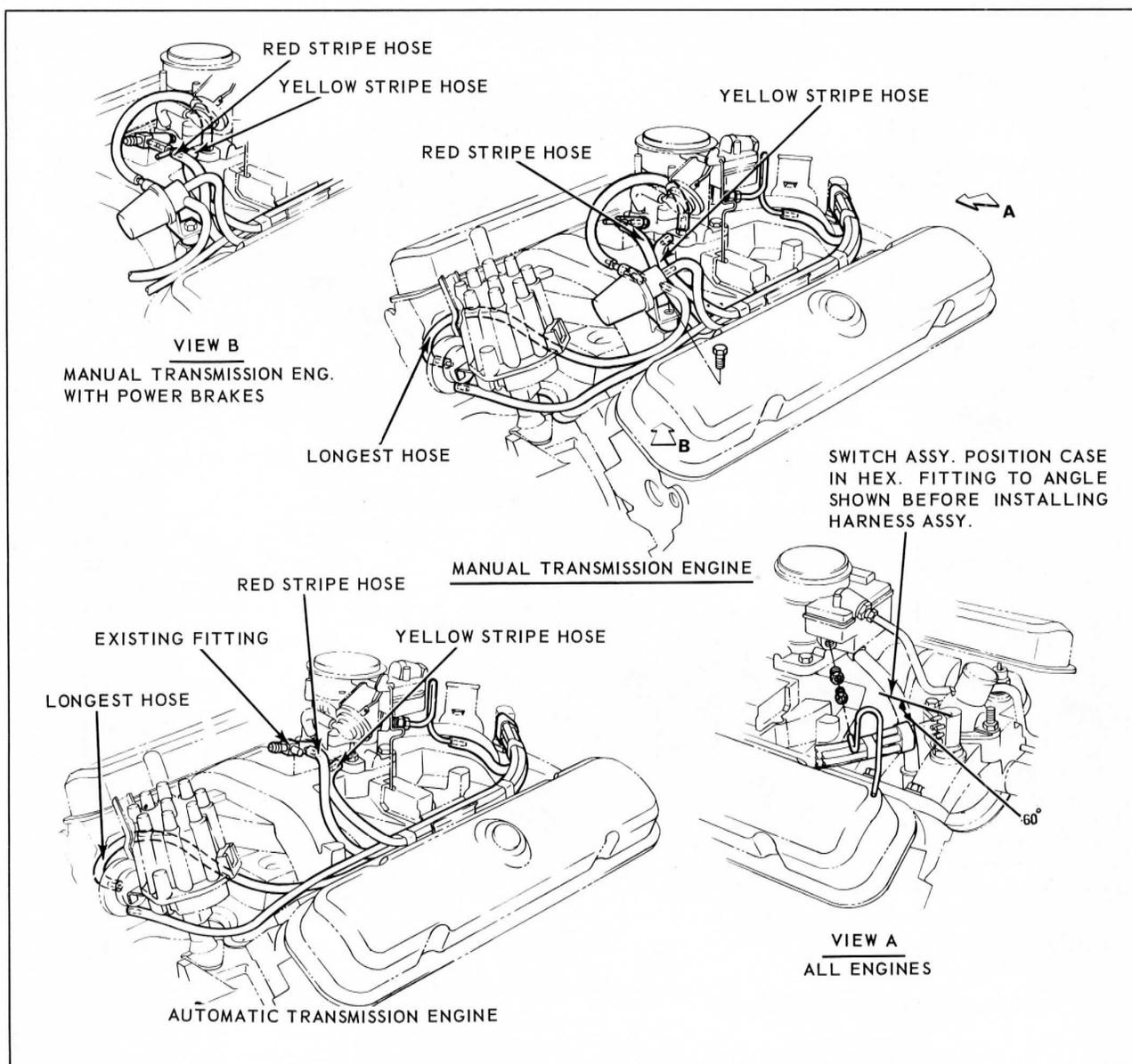
Fig. 6D-10 Distributor Vacuum Layout V-8 2 Bbl.
